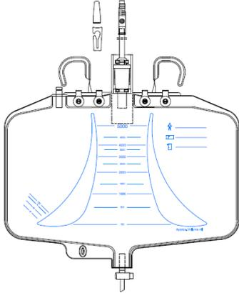
A technical diagram of a urine collection bag (REF 114541). It has a central inlet tube with a blue slide clamp, two side handles, and a Pasteur drip chamber integrated into the top inlet. A hydrophobic filter is inside. A needle-free sampling port with a protective cap is on the right. A T-tap drain valve is at the bottom. Blue lines indicate internal components and flow.                                    |
