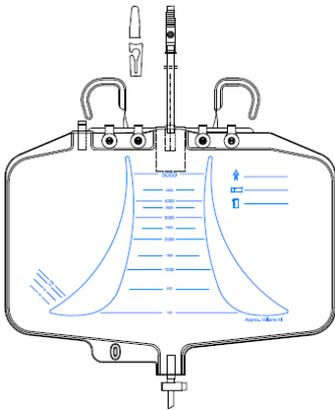
A technical diagram of a urine collection bag (REF 114543). It features a central inlet tube with a blue slide clamp and two side handles for bag hangers. A hydrophobic filter is inside. A needle-free sampling port with a protective cap is on the right. A T-tap drain valve is at the bottom. Blue lines indicate internal components and flow.                                                                       |
